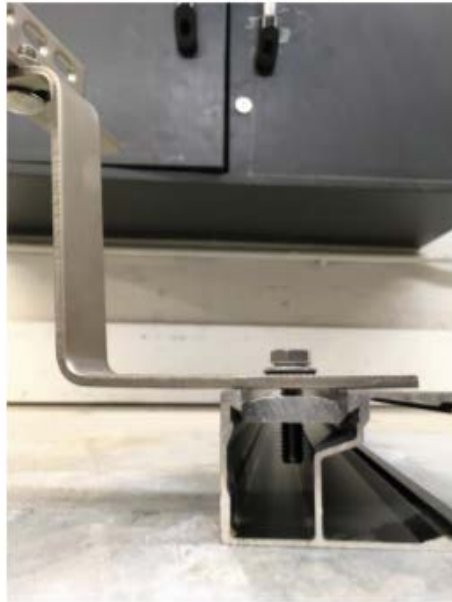
Figure B2b. Side view of connection
