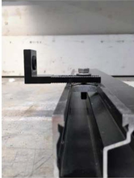
Figure B3b. Side view of connection
