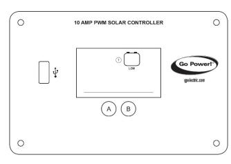
If the battery voltage reaches 11 volts, the battery SOC symbol will show the text "LOW" beneath it. The controller will continue operating in this condition and will only stop operating if the voltage drops below 9 volts.
