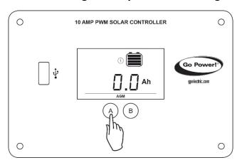
To reset the count of ampere hours charged, toggle to the ampere hours charged. Press and hold the **A Button** for 6 seconds to reset the counter to zero.
