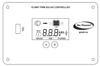
If the GP-PWM-10-FM experiences a battery over voltage (15.5V), the controller will stop operating, and the display will begin to flash with all icons. The controller will resume operating when the error is cleared.
