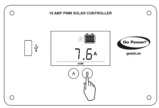
Push the **B Button** to show the PV charging current.
