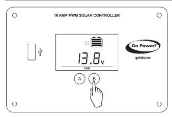
Push the **B Button** to show the battery voltage.
