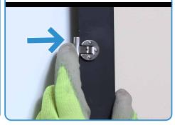
Align mounting slot and slide onto Set Clip until end is 6 inches past frame.
