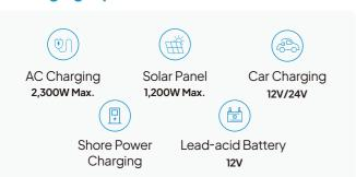
Note: Shore power charging: An extra adapter cable is required. How to connect: shore power outlet → adapter cable → charging inlet of AC240P.
