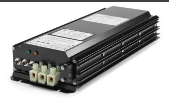
Model 6958 is designed to meet the emerging need to charge lithium battery banks from 12V systems. Model 6958 will output 22A @ 58V in full charge mode and can be operated while load is drawn from the battery bank being charged. Off the shelf units are ideal for use with lithium iron phosphate batteries. Model 6958 is microprocessor controlled and can be programmed at the factory for operation with other battery types.
